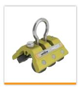
WT UniRail carriage (Part code: 7241027) – the carriage is part of the Unirail system. It provides a mobile attachment point for users to connect to. One user per carriage. Use only on straight systems. Minimum strength 22kN (5,000lbs)
