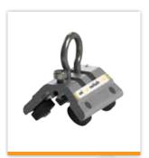
Attachment carriage (Part code: 7241006) – enables the user to connect to the system and enjoy complete hands-free movement along the rail. It features a stainless steel parking lock for work positioning tasks and aluminium, nylon coated wheels. A stainless steel shackle enables connection of a karabiner hook and pivots to enable best functionality at any angle of take off. Min strength 15kN (3300lbs)
