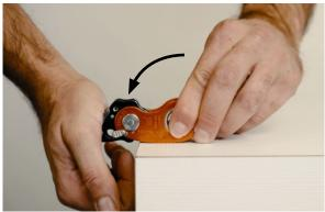
Use one hand to hold the device by the connection hole. With the other hand, rotate the cam outward and press down firmly with the palm. Finally, release the cam.
