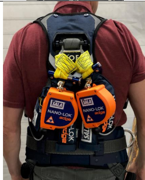
Figure 3 (photo of two Nano-Lok™ Edge Single-Leg Self Retracting Lifeline units attached to the dorsal D-ring with two Nano-Lok™ Edge Web Loop Harness Adaptor PN; 3500046)
