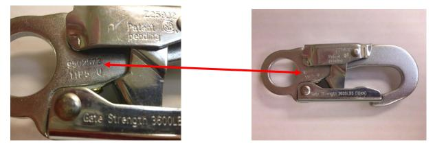
The recall includes all lanyards manufactured with snaphook # 9502573 between the manufacturing dates set out below. Manufacture date is marked on the product label of each lanyard as: **MFRD (YR/MO)**
