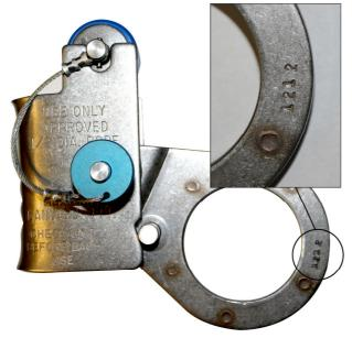
Due to an error during the manufacture of the rope grabs with SN#s listed above the rope grabs will not work and fail in case of an emergency.
